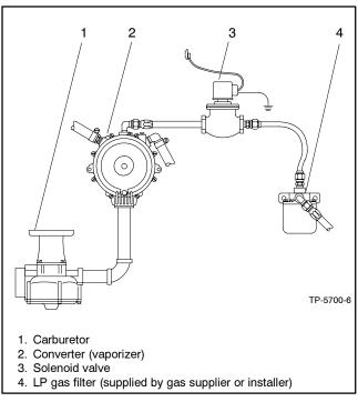
Figure 6-7 LP Gas Liquid Withdrawal System
